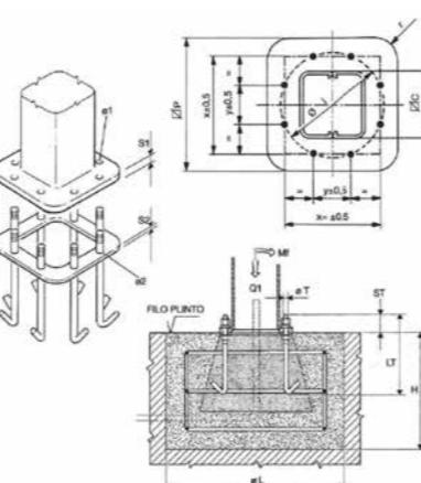
N.B.: The foundation frames with lug bolts, used in the column-mounted version for fixing the column itself to the foundation plinth is supplied on request.
