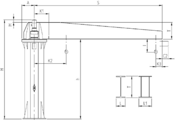
GBR jib cranes with DRH electric wire rope hoist:
