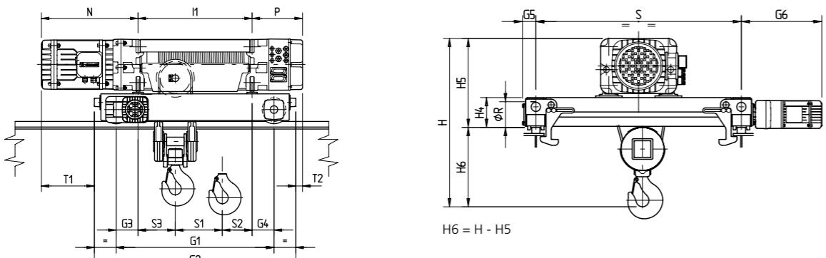
(\*) The standard gauge is S=1000 mm, a gauge of S = 1200 mm can be supplied upon request
