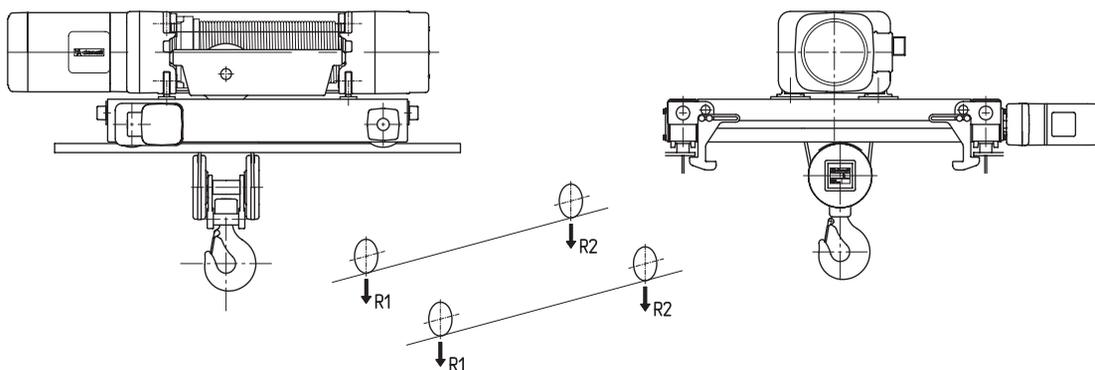
**CHARIOTS BIPOUTRE DRT POUR PALANS ELECTRIQUES A CABLE DRH - VERSION PERPENDICULAIRE A 2 BRINS (2/1) ET A 4 BRINS (4/1)**
