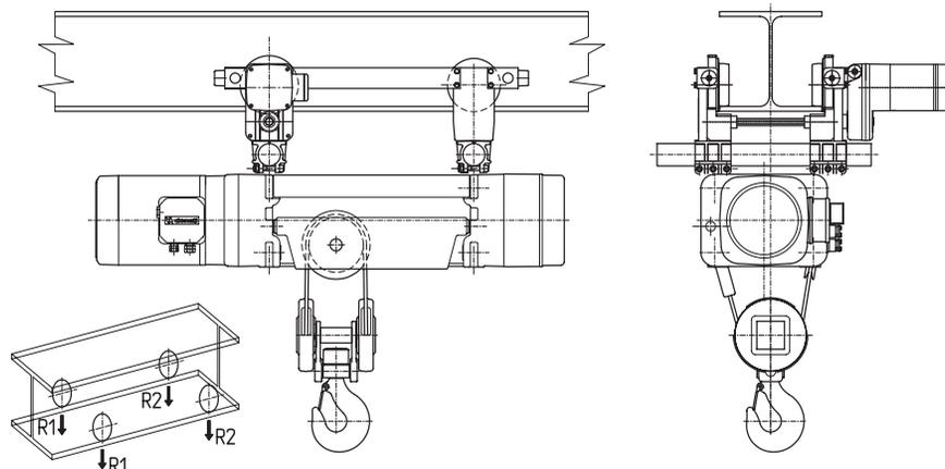
**CHARIOTS MONOPOUTRE DST/R POUR PALANS ELECTRIQUES A CABLE DRH - VERSION A 2 BRINS (2/1)**
