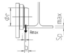
\* Max R calculated with a dynamic coefficient of 1.15 and no "M" increasing coefficient
